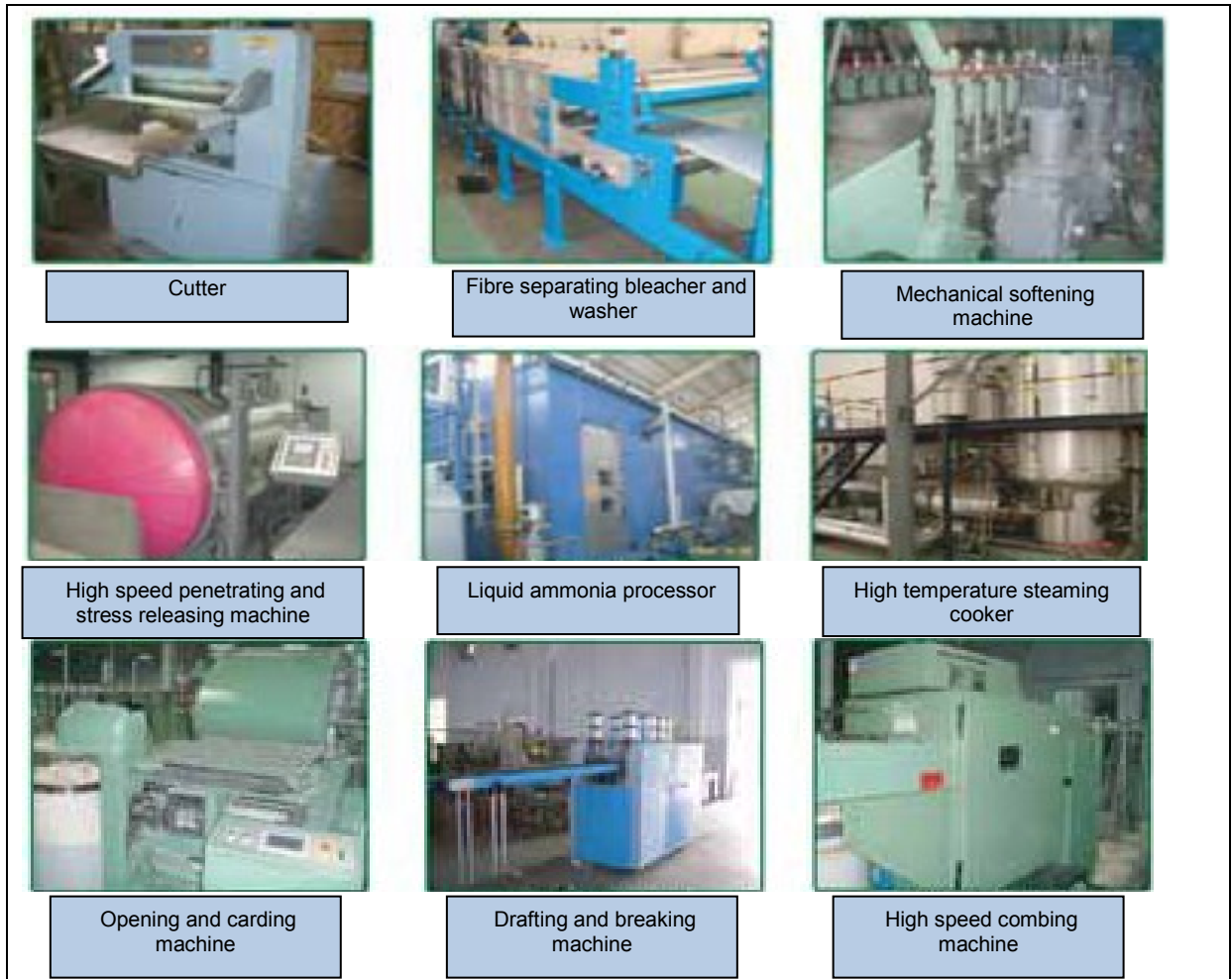
Exhibit 6.3.12: Machines developed for cottonisation of hemp in China
